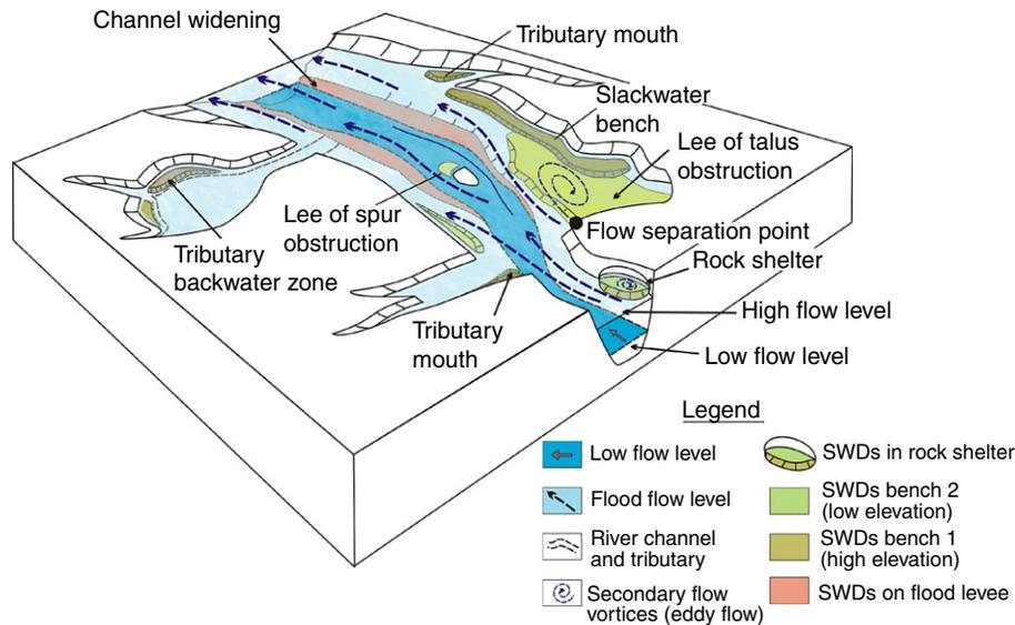
**Figure 2** Block diagram illustrating the location of sedimentary environments related to flood deposition. Modified from Benito, G., Sánchez, Y., Sopeña, A., 2003b. Sedimentology of high-stage flood deposits of the Tagus River, Central Spain. *Sedimentary Geology* 157, 107–132.
